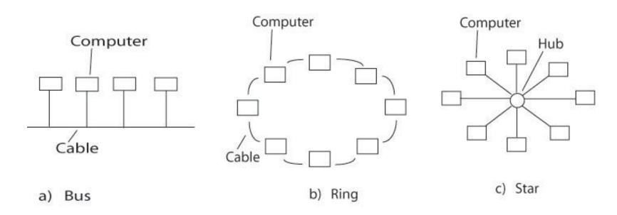
Figure: Topologies commonly used in LANs.
